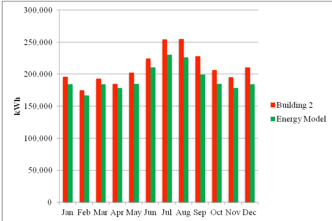
Figure 5, Building 2 Electricity vs. Model
